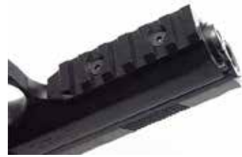
#- " h k Aluminum accessory rail for the 97B. CNC machine from Billet Aluminum. Frame requires drilling and tapping. Supplied with 2 x M4 x 0.7 Screws. BLACK | SKU: #10274
